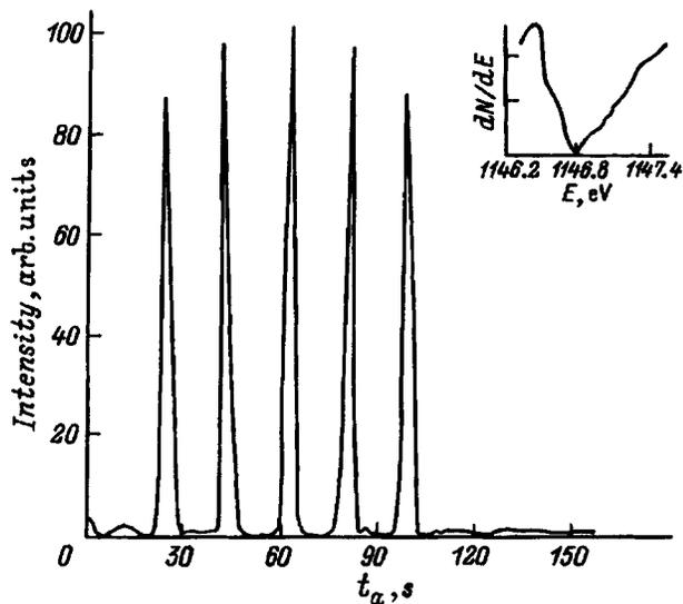
FIG. 3. Variation in the intensity of the Ge Auger peak  $E=1146.8$  eV with layerwise etching of the surface of a strained  $\text{Si}_{1-x}\text{Ge}_x$  superlattice by Ar ions. The ion energy is 2.8 keV, the current is  $250\mu\text{A}/\text{cm}^2$ , and the ion beam diameter is  $0.75\mu\text{m}$ . The period of the superlattice is  $160\text{Å}$ . Inset: Ge Auger peak.
