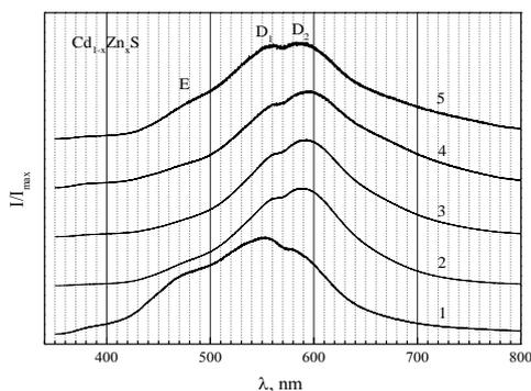
**Fig. 5** – PL spectrum of  $\text{Cd}_{1-x}\text{Zn}_x\text{S}$  NCs at  $T = 300$  K. The line number corresponds to the following samples listed in Table 1: 1 – Cd100; 2 – Zn25; 3 – Zn50; 4 – Zn75; 5 – Zn100
