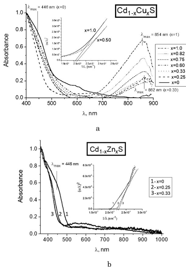
Fig. 2 – Absorption spectra of polymer films with embedded NCs of  $\text{Cd}_{1-x}\text{Cu}_x\text{S}$  (a) and  $\text{Cd}_{1-x}\text{Zn}_x\text{S}$  (b). Tauc's plots in coordinates  $(\alpha\lambda)^2$  vs.  $1/\lambda$  are shown in insets
