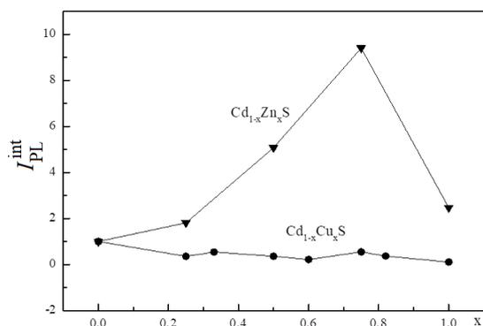
**Fig. 6** – The effect of nanocrystal composition of semiconductors  $\text{Cd}_{1-x}\text{Cu}_x\text{S}$  and  $\text{Cd}_{1-x}\text{Zn}_x\text{S}$  on the intensity of their integrated PL
