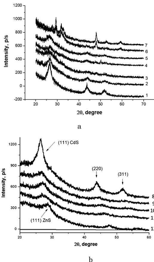
**Fig. 3** – XRD patterns of NCs of  $\text{Cd}_{1-x}\text{Cu}_x\text{S}$  (a) and  $\text{Cd}_{1-x}\text{Zn}_x\text{S}$  (b) with different compositions. The pattern number corresponds to the following samples listed in Table 1: 1 – Cd100; 2 – Cu33; 3 – Cu50; 4 – Cu60; 5 – Cu75; 6 – Cu82; 7 – Cu100; 8 – Cd100; 9 – Zn25; 10 – Zn50; 11 – Zn75; 12 – Zn100
