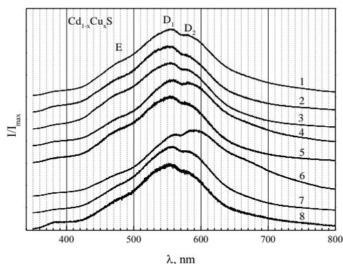
**Fig. 4** – PL spectra of  $\text{Cd}_{1-x}\text{Cu}_x\text{S}$  NCs at  $T = 300$  K. The line number corresponds to the following samples listed in Table 1: 1 – Cd100; 2 – Cu25; 3 – Cu33; 4 – Cu50; 5 – Cu60; 6 – Cu75; 7 – Cu82; 8 – Cu100
