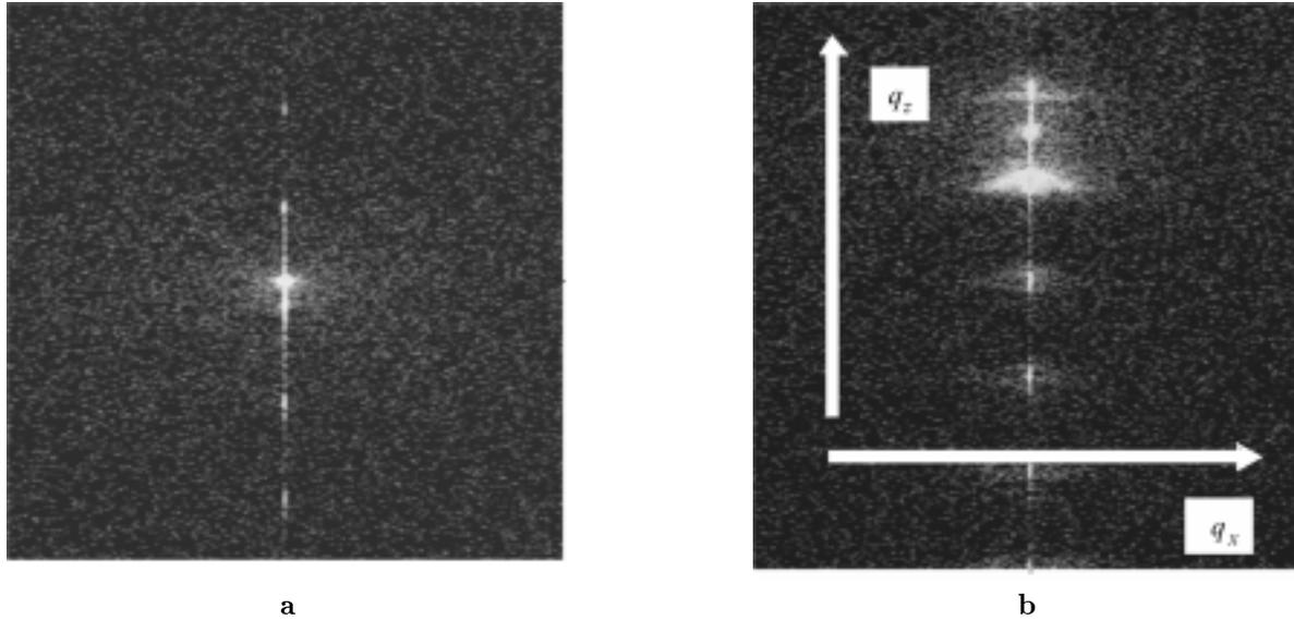
Fig. 2. Reciprocal space distribution maps of the diffracted intensity around a symmetric 004 point in the SiGe/Si structures with 4- (a) and 7-ML (b) Ge layers.  $\text{CuK}\alpha_1$  emission
