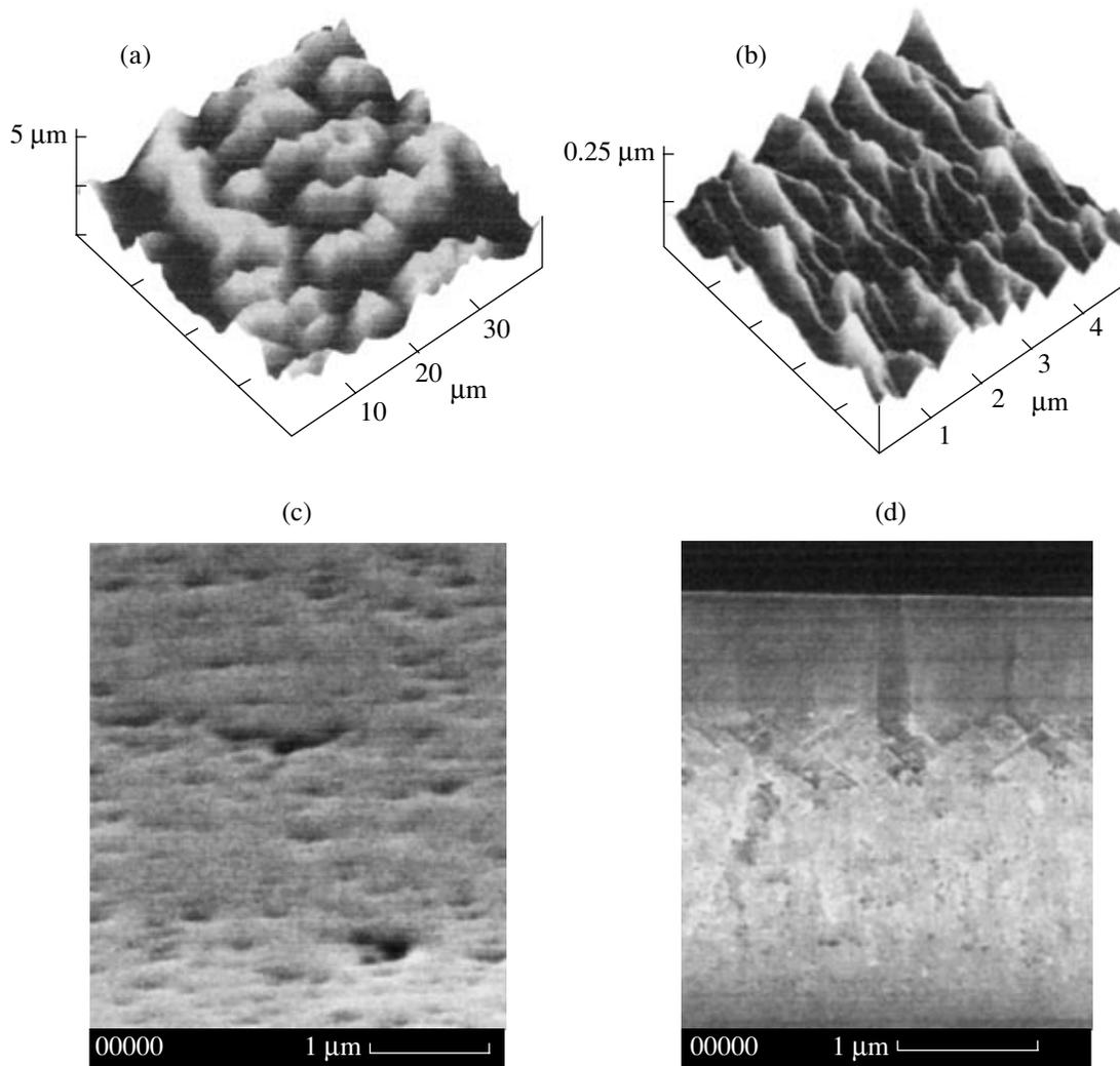
**Fig. 1.** (a), (b) AFM and (c), (d) SEM images of GaAs microprofile surfaces of (a) dendrite and (b) quasi-grating types; (c) GaAs porous layer; and (d) cross section of the epitaxial layer on a porous GaAs substrate.
