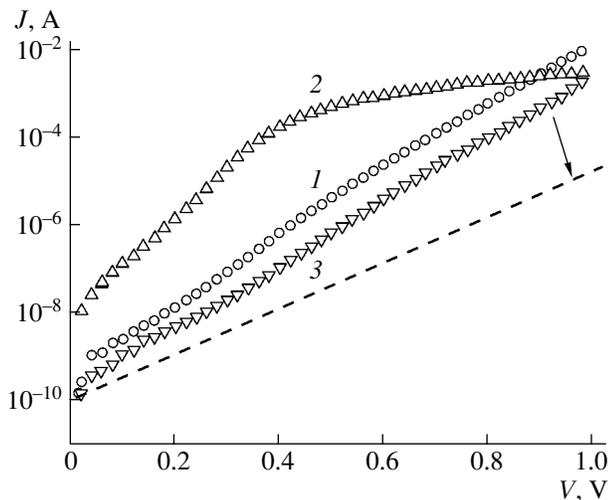
**Fig. 5.** Forward  $I$ - $V$  characteristics in the dark for photovoltaic converters based on LPE-structures on: (2) smooth surface, sample LPE-144; (1) and (3), microprofile substrates of quasi-grating type, samples LPE-143 and LPE-145, respectively. Dashed line, the simulated characteristic for a sample on porous substrate with the dislocation density in the layer of  $10^3 \text{ cm}^{-2}$ . The arrow indicates the shift of this line as the technology of epitaxy is optimized.
