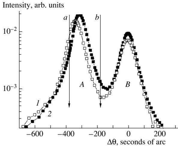
**Fig. 2.** X-ray rocking curves ((004) reflection,  $\text{CuK}\alpha$  radiation) for MOCVD-structures on (1) smooth and (2) profiled surfaces of GaAs substrate. A and B, peaks of reflection from  $\text{Al}_{0.8}\text{Ga}_{0.2}\text{As}$  epitaxial film and GaAs substrate, respectively; (a) and (b), peak positions for completely stressed and completely relaxed structures, respectively.
