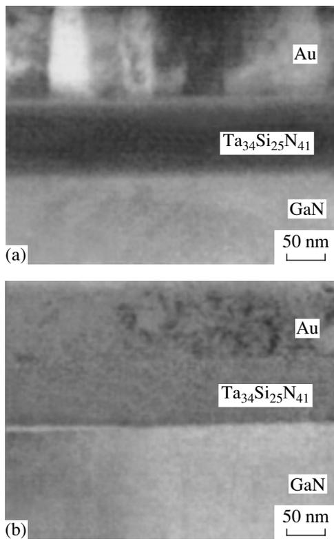
**Fig. 3.** TEM micrographs taken of the cross section of the Au/Ta<sub>34</sub>Si<sub>25</sub>N<sub>41</sub>/GaN samples (a) as-deposited and (b) annealed at 800°C for 5 min in the Ar flow.
