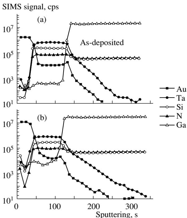
**Fig. 2.** SIMS element distributions over the depth in the (a) as-deposited Au/Ta<sub>34</sub>Si<sub>25</sub>N<sub>41</sub>/GaN contact structures and (b) the same structures annealed at 800°C for 5 min in the Ar flow.
